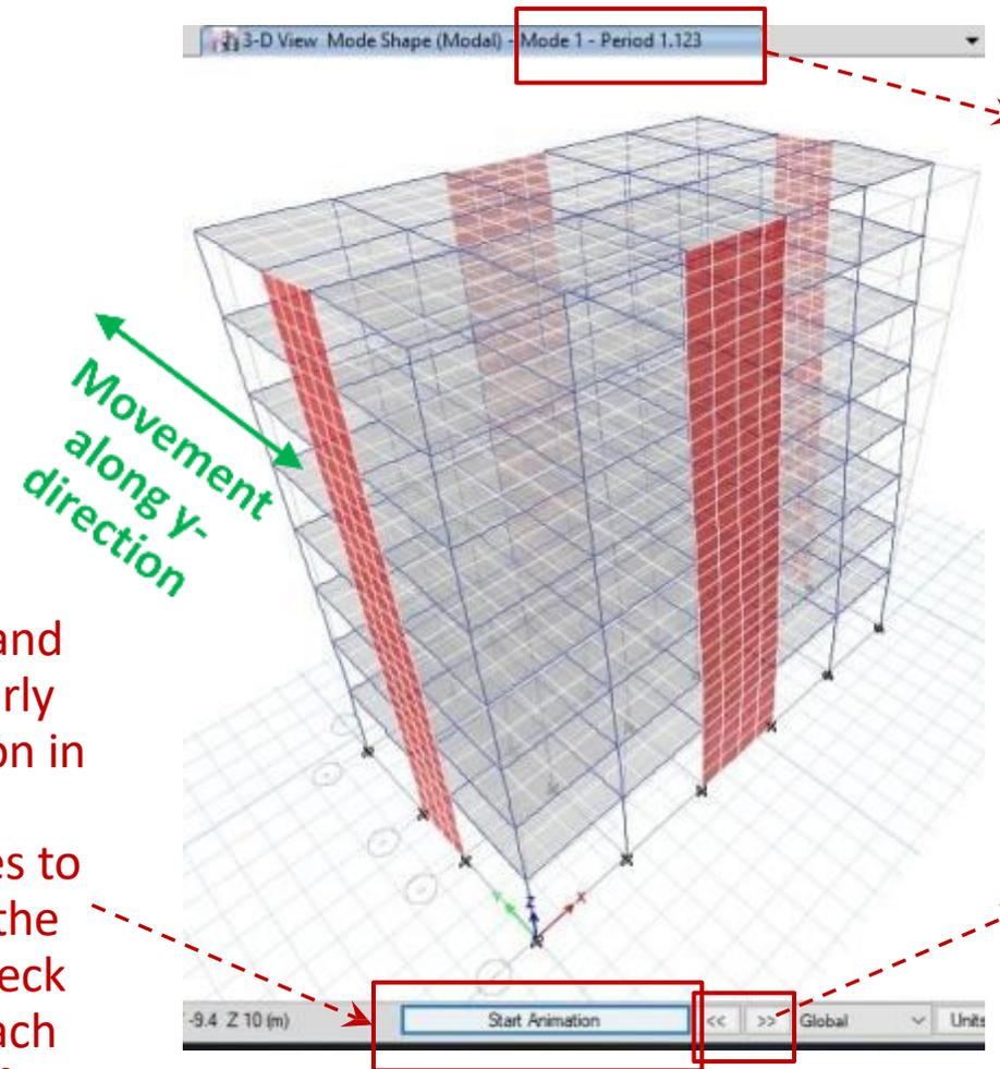
Now that we understand that the first mode corresponds to the lateral movement along y-direction, this value becomes to be our fundamental period along this direction.  $T_1^{(y)}=1.123$  sec.
