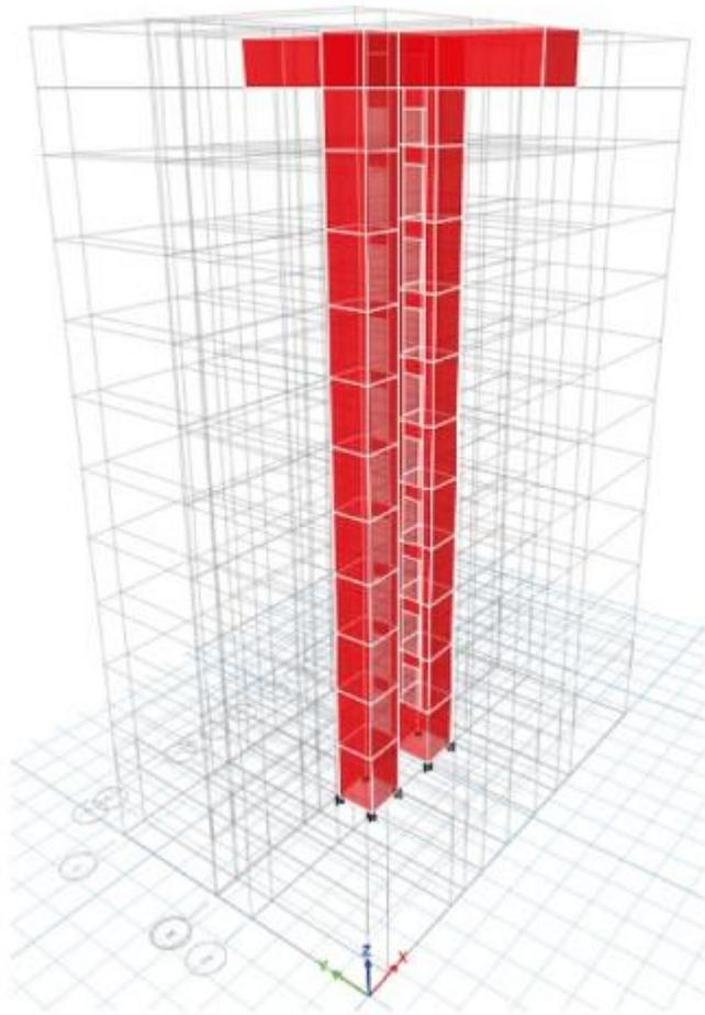
Shear Wall Design with Boundary Element, Spandrel or Coupling Beam
