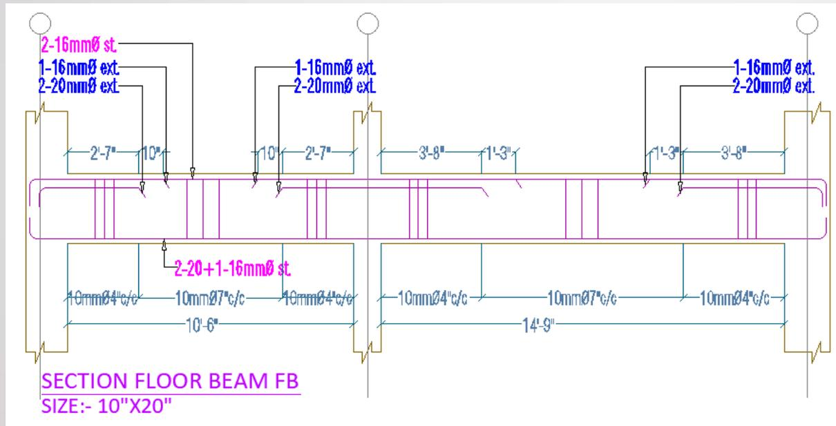
**Provided Area of Rebar for Beam**
