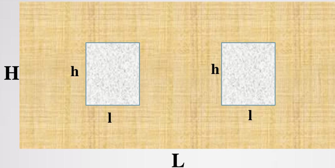
Wall Load = Equivalent Height of Wall X Weight Per Unit Area of Wall
