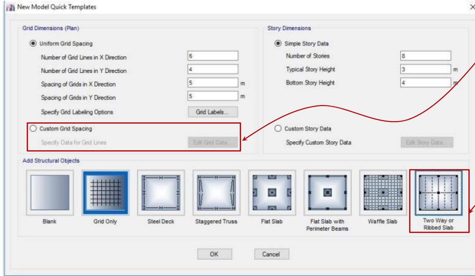
Next select «Custom Grid Spacing» and click here (Edit Grid Data) to make the correction for the only span length of 3 m (shown in the next slide)!
