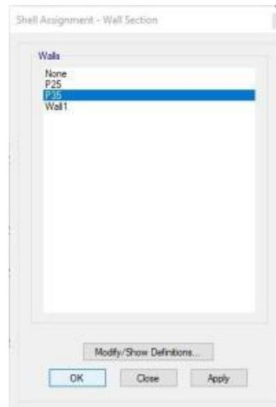
Do the same operations to select the shear walls at the upper similar stories (stories 3-4-5 and 6-7-8) and assign «P25» wall section to your selection. Now that we have finished assignment of all shear wall sections.
