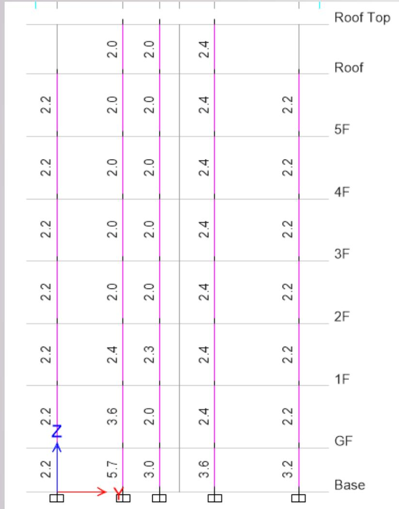
Require Area of Rebar (in<sup>2</sup>) for Column
